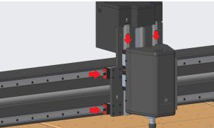
First home the machine, then move the X axis 24" to the right and the Y axis 10" to the back for easy access to the grease points. Then open the grease gun packaging and assemble the gun as shown in the picture below. Pump the grease gun until you see grease come out of the nozzle. Push the nozzle firmly against the grease nipple in the guide block, squeeze the black tube, and pump the grease gun a few times until you see grease ooze out of the sides of the guide blocks.
